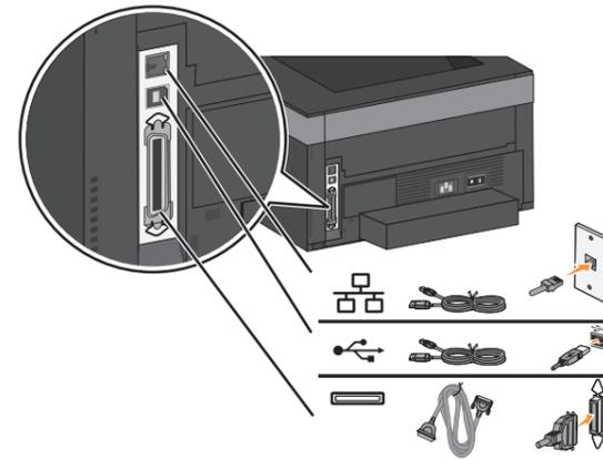
Connect the printer to a computer using a USB or parallel cable, or to a network (2330dn and 2350dn only). Cables are sold separately.
